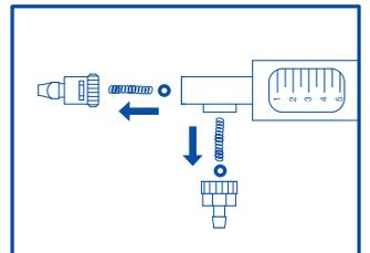
If insufficient, disassemble valves and clean.
