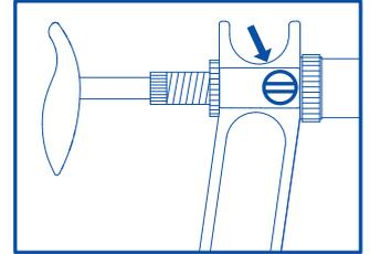
Adjust body / grip position using locking screw on handle side.
