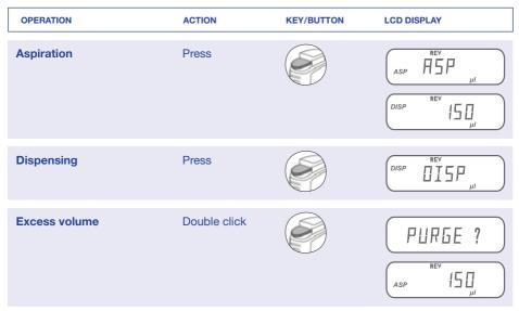
**Notes:** Skip "purge" by holding start button down after dosing is completed. The next sample is aspirated directly after release of the start button. Slightly touch reservoir wall when dispensing.
