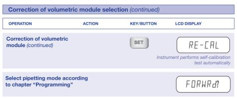
Note: WARNING, the programmed volumetric module must correspond to the one fitted on the pipette assembly.
