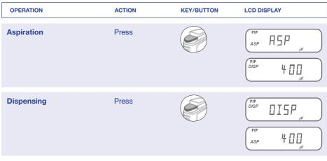
**Notes:** Plunger stays down when start button is kept pressed, and returns to initial position when released. Slightly touch reservoir wall when dispensing.
